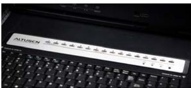
In addition to the powerful, menu-driven OSD, port switching can be quickly and conveniently carried out by pressing push-button
