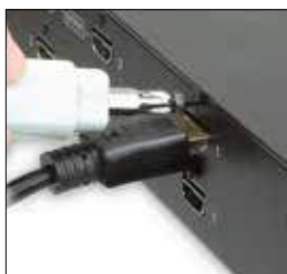
Loosen the screw above the port
