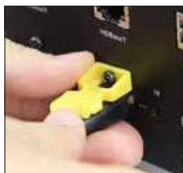
Slide the LockPro over the loosened screw
