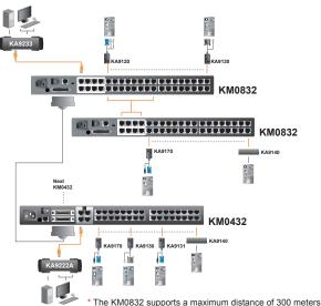
\*The KM0832 supports a maximum distance of 300 meter between console modules and KVM adapter cables.
