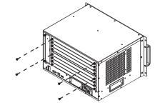
3. Slide the I/O board into the open slot on the VM1600 until it secures in place.
