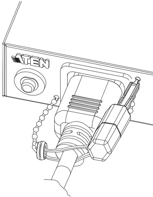
5. Slide the left and right rings of the Cable Holder towards the middle so that the power cord is completely fastened to finish.
