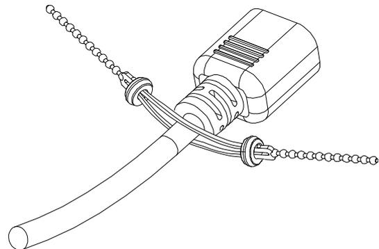
2. Plug the power cord into the PDU's power outlet, and thread one end of the Lok-u-Plug Cable Holder into the lower left hole next to the power outlet.
