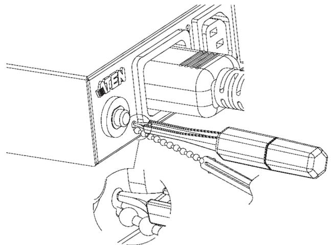
4. Push the Cable Holder as close to the PDU as possible. Then thread its other end to the upper right hole next to the power outlet, and lock it in place using the Installation Tool by repeating step 3.
