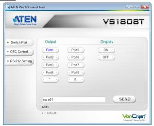
The Switch Port page is used to power on or power off the display connected to a port.
