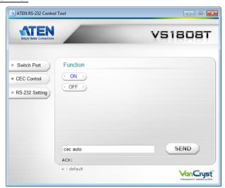
The CEC Control page is used to enable or disable the CEC Control feature. The default setting for the CEC Control is off.
