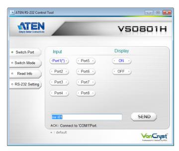
The Switch Port page is used to connect a source device to the display port, and to power the display port On/Off. On the Switch Port page, the following actions are possible:
