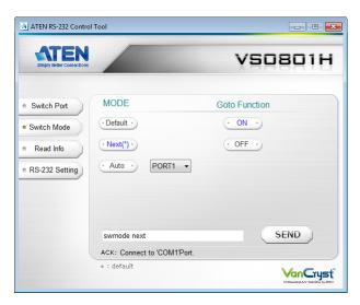
You can choose how the VS0801H behaves when a new input source is connected to it. By default the Next switch mode setting is enabled. Use the commands below to select a different mode. There are three Switch Modes:
