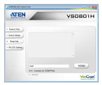
The read command allows you to read information about the connected device. Click **Send** to retrieve information.
