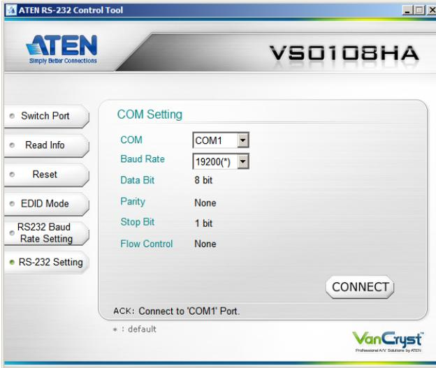
The controller's serial port should be configured as follows:
