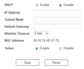
**Enable** DHCP to allow the DHCP server to assign an IP address to the VM1600A. Select **Disable** to enter your own static IP address settings for the device.
