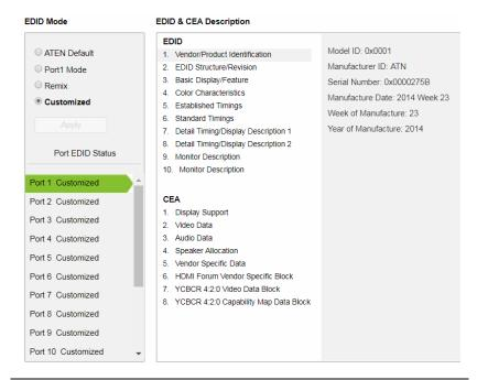
**Note:** The EDID Mode can also be selected via the Front Panel pushbuttons – see *Operation Mode*, page 55.
