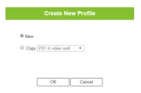
Select New to create a new profile or Copy to use configuration from a pre-existing profile. This screen appears.
