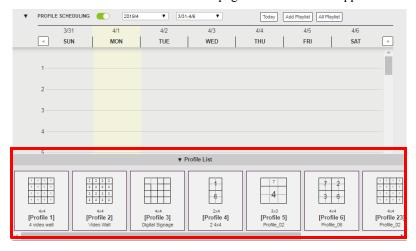
4. From the Profile List, drag and drop profiles onto the desired time on the calendar view. Optionally right-click the profile to copy, remove, or view its settings.
