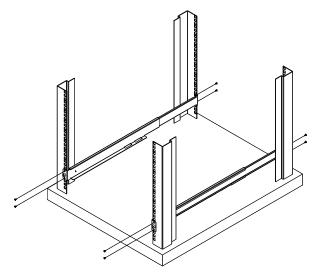
2. Slide the unit along the brackets, then screw the front panel to the rack.
