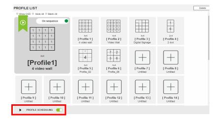
**Note:** For firmware prior to version 4.2.416, if profile scheduling is disabled and re-enabled within the scheduled time frame of a playlist, the VM1600A will resume playing the first profile in the playlist; for VM1600A of firmware version 4.2.416 or later, the system will resume playing the playlist according to schedule, and the profiles that were to be played during the paused period will be skipped.
