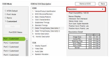
In the drop down menu, choose a resolution with values that fit the attached monitor/display device and click **Save**.
