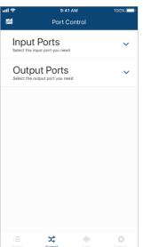
In the **Control** tab, you can instantly switch video inputs for each of the output.
