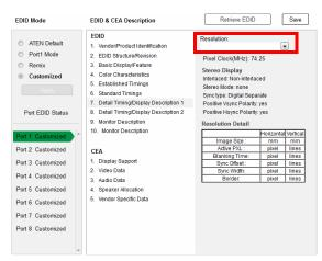
In the drop down menu, choose a resolution with values that fit the attached monitor/display device and click **Save**.
