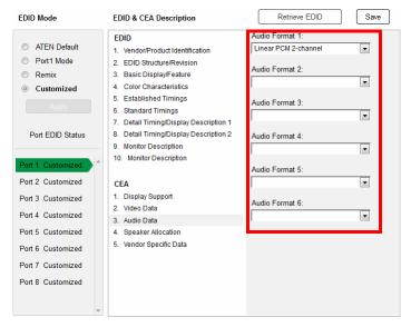
Use the drop down menu to select the **Audio Format** ( $1\sim6$ ) applicable to your audio output device, and click **Save** to apply the changes.
