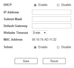
**Enable** DHCP to allow the DHCP server to assign an IP address to the VM0808HA. Select **Disable** to enter your own static IP address settings for the device.
