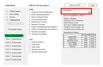
In the **Resolution** drop down menu, choose a resolution with values that fit the attached monitor/display device and click **Save**.
