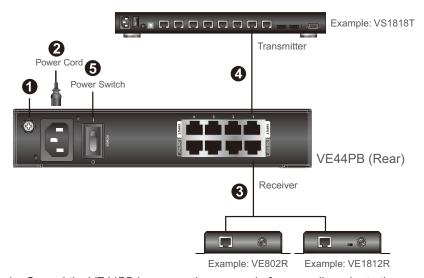
Ground the VE44PB by connecting one end of a grounding wire to the grounding terminal and the other end to a suitable grounded object.
