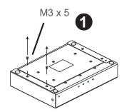
Use the screws from step 1 to screw the mounting bracket on the bottom of the VF44PB.
