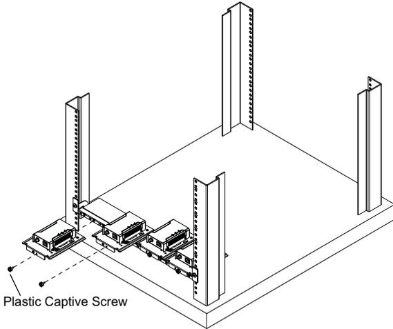
For a device that aligns to line B, you can install up to 3 units:
