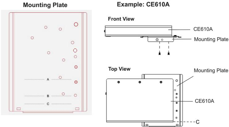
b) Secure the device to the mounting plate from the backside using the supplied countersunk head screws.
