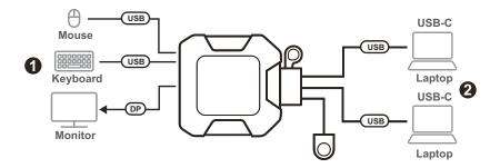
1. Connect the USB mouse, USB keyboard, and DisplayPort monitor into their respective ports on the US3312.
