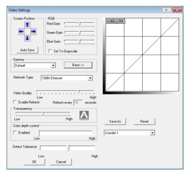
This section allows you to adjust the video display's gamma level.
