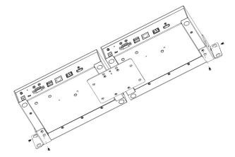
4. Screw the mounting brackets to the rack.
