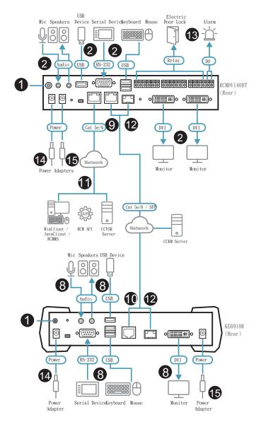
**Note:** The diagram above shows the RCMDVI40BT setup with a KE6910R. The RCMDVI00AT-KE6900AR installation is the same except with one less DVI monitor.
