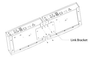
3. Remove the bottom and side screws from each unit.
