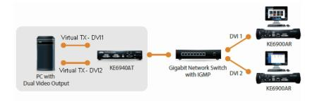
When connecting to either of the two Virtual Transmitters in the setup shown above, the mouse cursor may reside on the **main** or **extended** dual display screen, out of view. Therefore even if you have control of the mouse it may not be visible. To bring the mouse cursor into view on either of the dual display screens, first, enable Boundless Switching (see *Boundless Switching*, page 138) and then use the hotkey **F8+F9**.
