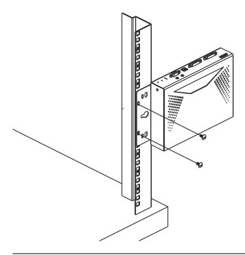
**Note:** Rack screws are not provided. We recommend that you use M5 x 12 Phillips Type I cross recessed screws.
