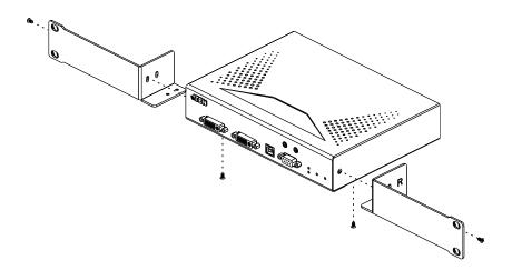
4. Screw the mounting brackets to the rack.
