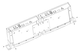
5. Screw the mounting brackets to the rack.
