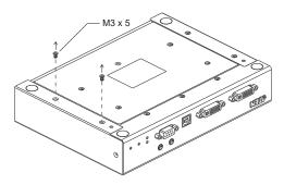
2. Use the screws from step 1 to screw the mounting bracket to the bottom of the Transmitter as shown below:
