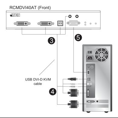
**Note:** The serial port on the transmitter (shown above) connects to the computer; the serial port on the receiver (not shown) connects to a serial device (optional).
