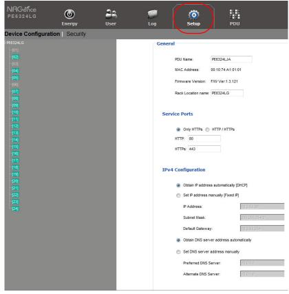
3. Fill in the **IPv4 Configuration** fields according to the information provided under *IPv4 Configuration*, page 42.
