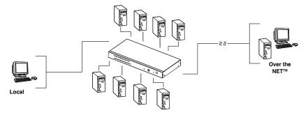
In addition to TCP/IP connectivity, the KH1508i / KH1516i provides KVM ports for a locally attached PS/2 console – allowing access and control from the data center as well as over the Net. The switches utilize a single shared bus implementation – although they support local and remote login at the same time, they do not support independent operation. If a local user logs in while a remote user has already opened a session, the local user sees the same screen that the remote user is working on.
