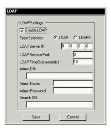
To allow authentication and authorization for the KH1508i / KH1516i via LDAP / LDAPS, set the parameters as follows:
