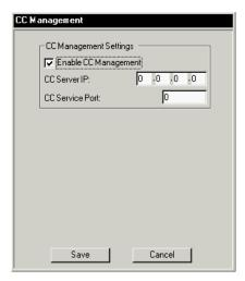
To allow authorization for the KH1508i / KH1516i through a CC (Control Center) server, check *Enable* and fill in the CC Server's IP address and the port that it listens on in the appropriate fields.
