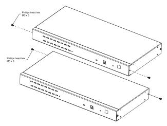
2. Screw the mounting brackets into the sides of the unit at the front or the rear, as shown in the diagram below.
