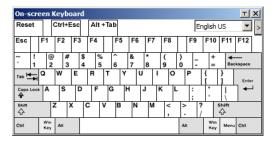
One of the major advantages of the on-screen keyboard is that if the keyboard languages of the remote and local systems aren't the same, you don't have to change the configuration settings for either system. The user just has to bring up the on-screen keyboard; select the language used by the computer on the port he is accessing; and use the on-screen keyboard to communicate with it.
