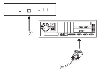
**Note:** On a daisy chained installation, connect the cable to the first station (master) unit. The chained stations (slaves) will receive the upgrade via the daisy chain cables.
