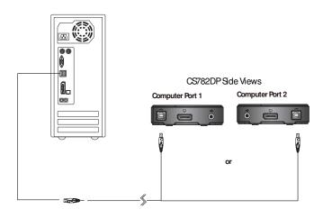
3. The CS782DP now enters Firmware Upgrade Mode. The two Ports LEDs flash together to indicate that the unit is in Firmware Upgrade Mode.
