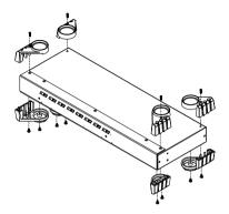
2. Use the screws that came with the rack mount kit to screw the mounting brackets into the sides of the unit, as shown in the diagram below:
