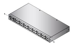
2. Use the M3 x 6 Phillips hex head screws supplied with the rack mounting kit to screw the rack mounting brackets into the sides near the rear of the unit.
