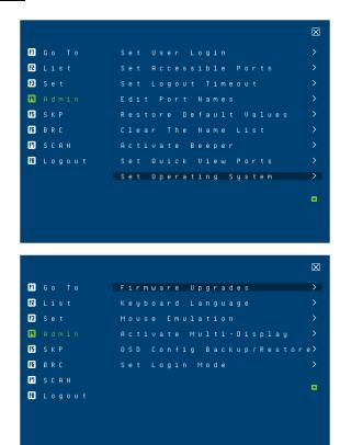
Clicking Admin or pressing [F4] activates Admin function. F4 is an administrator only function. It allows the administrator to configure and control the overall operation of the OSD. To change a setting, click on the settings item you want to configure, or use the up and down arrow keys to move the highlight bar to it then press [Enter].
