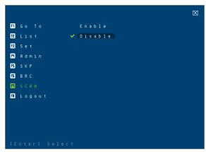
Clicking SCAN or pressing [F7] invokes *Auto Scan* mode. This function allows you to automatically switch among the available computers at regular intervals so that you can monitor their activity without having to take the trouble of switching yourself. Enable mouse emulation for Auto Scan to work (see page 41).
