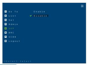
Clicking S K P or pressing [F5] invokes Skip (SKP) mode. This function enables you to easily skip backward or forward – switching the console focus from the currently active computer port to the previous or next accessible one. Enable mouse emulation for Skip mode to work (see page 41).
