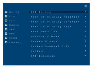
Clicking E set or pressing [F3] activates the Set function. This function allows the administrator and each user to set up his own working environment. A separate profile for each is stored by the OSD and is activated according to the username that was provided during login.
