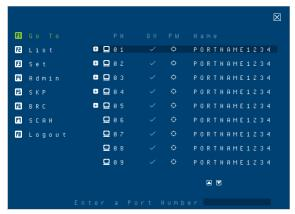
Clicking [f] G o T o or pressing [F1] activates the Go To function. Go To allows you to switch directly to a port by keying in the port's ID. Enable mouse emulation for independent switching (see page 41), for this function to work.
