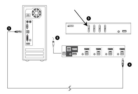
4. At the other end of the USB cable, connect the USB Type-B connector to the USB Type-B port in the port 1 KVM section.
