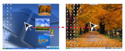
When the Cursor Shift is operated, the video output of the upper matrix window shifts between the two displays (and matrix windows) as shown above and described below:
