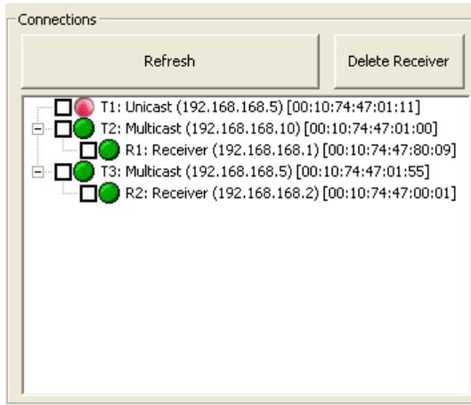
The *Connections* section displays the connections between the CE790T Transmitters and CE790R Receivers in the installation. It also displays basic configuration information for each unit – topology (Unicast or Multicast – Transmitters only); IP address; and Mac address.
