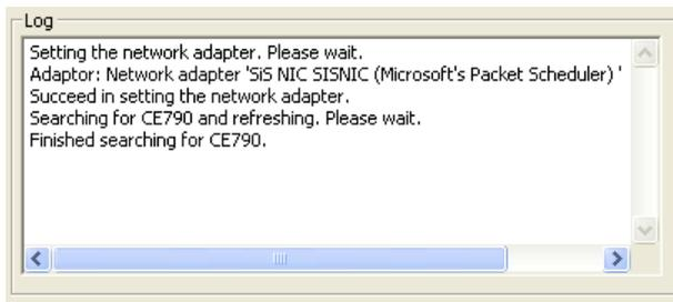
The *Log* section displays all the events that take place in the Browser GUI, in addition to displaying error messages.
