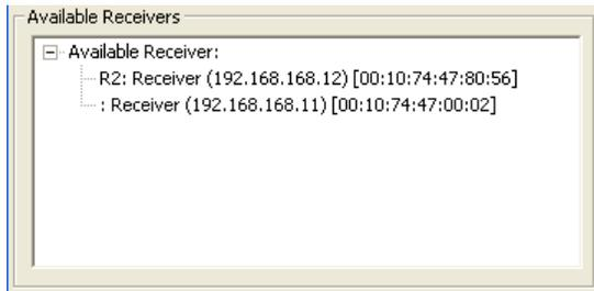
The *Available Receivers* section displays the CE790R Receivers that are currently attached to the installation and are available for connection. Select a CE790R Receiver in this list to view detailed information in the *CE790 Configuration* section. See *CE790 Configuration*, page 7.
