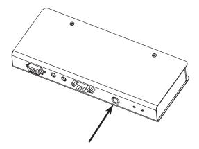
When you press the *Auto/Local* pushbutton and select **Local**, the Local LED lights solid green and the computer can only be accessed at the local console. In **Local** mode, the remote console cannot access the computer.
