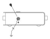
2. Be sure the computer and monitor connected to the CE770L/CE770RQ are properly grounded.
