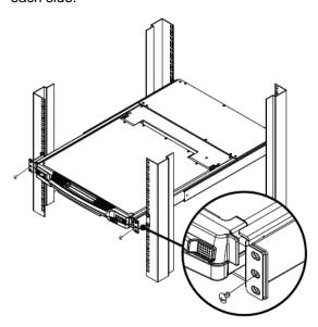
4. After the L-shaped brackets are secured, tighten all the screws. Allow at least 5.1 cm on each side for proper ventilation, and at least 12.7 cm at the back for the power cord and cable clearance.
