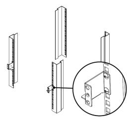
2. Attach the left and right L-shaped brackets to the back of the rack, installing four screws in the brackets to secure them in place.
