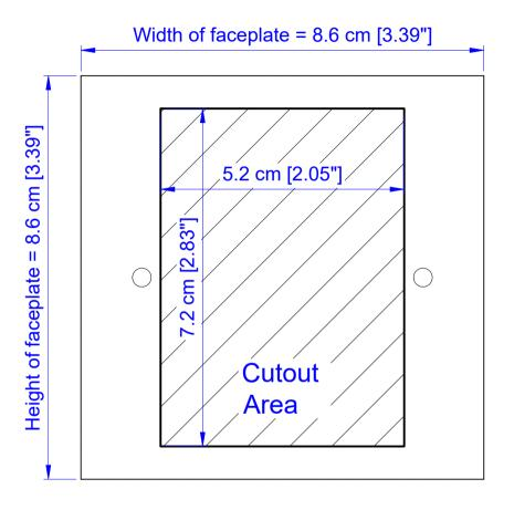
**Note:** ATEN recommends a 1-gang wall box with a depth of at least 5.5 cm (2.17 inches) to accommodate the connectors and cables.
