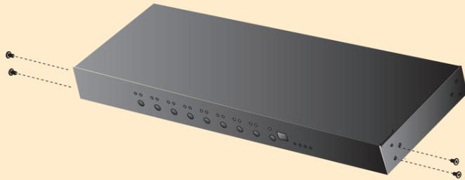
2. Screw the rack mounting brackets into the front and rear modules.
