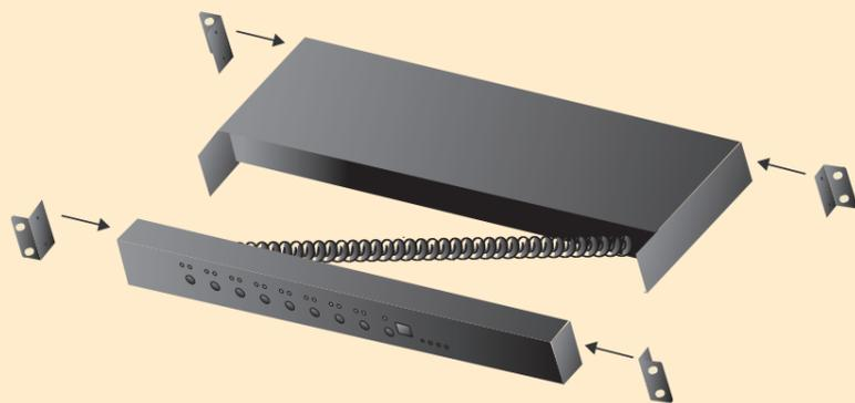
3. Screw the mounting brackets to the rack.
