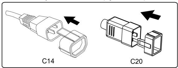
2. Insert the plug, with the EZ-Lok Plug Connector attached, into any available socket on a PDU by sliding it directly over and straight into the socket.
