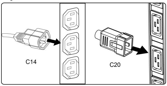
3. To disconnect the plug from the PDU, grip onto and squeeze the EZ-Lok Plug Connector as you pull and detach the plug from the PDU socket.
