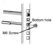
5. Insert the M6 nuts onto the support columns as show below:
