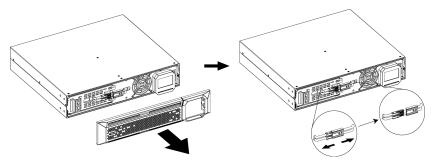
Remove the cover of the External Battery Connection Port using a screwdriver.
