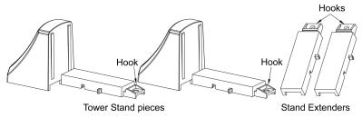
3. Orient the stand extenders as shown in the diagram below. Level and connect the extenders to the bottom of the tower stand pieces as indicated by the arrow. Make sure the hooks are properly hooked into the tower stand pieces.
