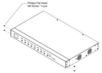
2. Use the screws you just removed, and the ones supplied with the rack mounting kit to screw the rack mounting brackets into both modules:
