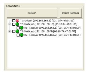
The *Connections* section displays the connections between the CE790T Transmitters and CE790R Receivers in the installation. It also displays basic configuration information for each unit – topology (Unicast or Multicast – Transmitters only); IP address; and Mac address.
