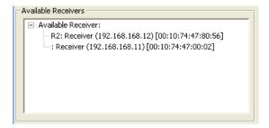
The *Available Receivers* section displays the CE790R Receivers that are currently attached to the installation and are available for connection. Select a CE790R Receiver in this list to view detailed information in the *CE790 Configuration*, page 7.
